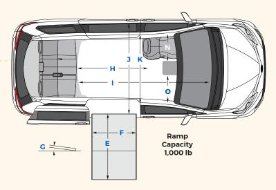
Seats up to seven passengers with an option for three wheelchairs. Seating options may vary depending on available payload.
