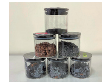
Materials recovered from recycled batteries
